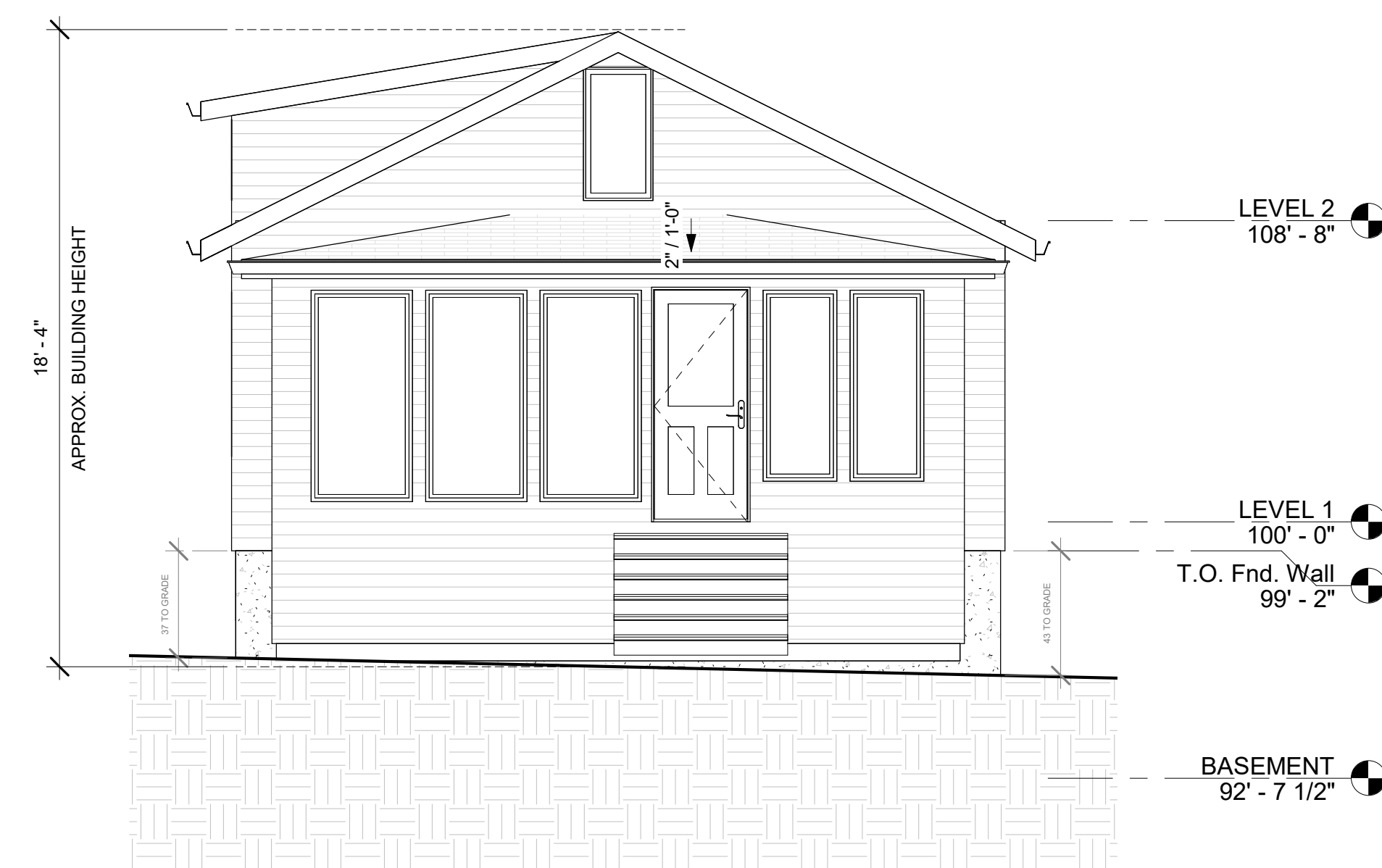
① SOUTH ELEVATION - AS-BUILT 1/4" = 1'-0"
