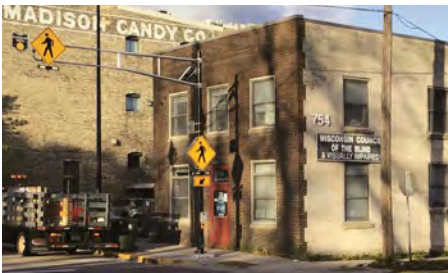
Rectangular rapid flashing beacon (RRFB) in Madison
