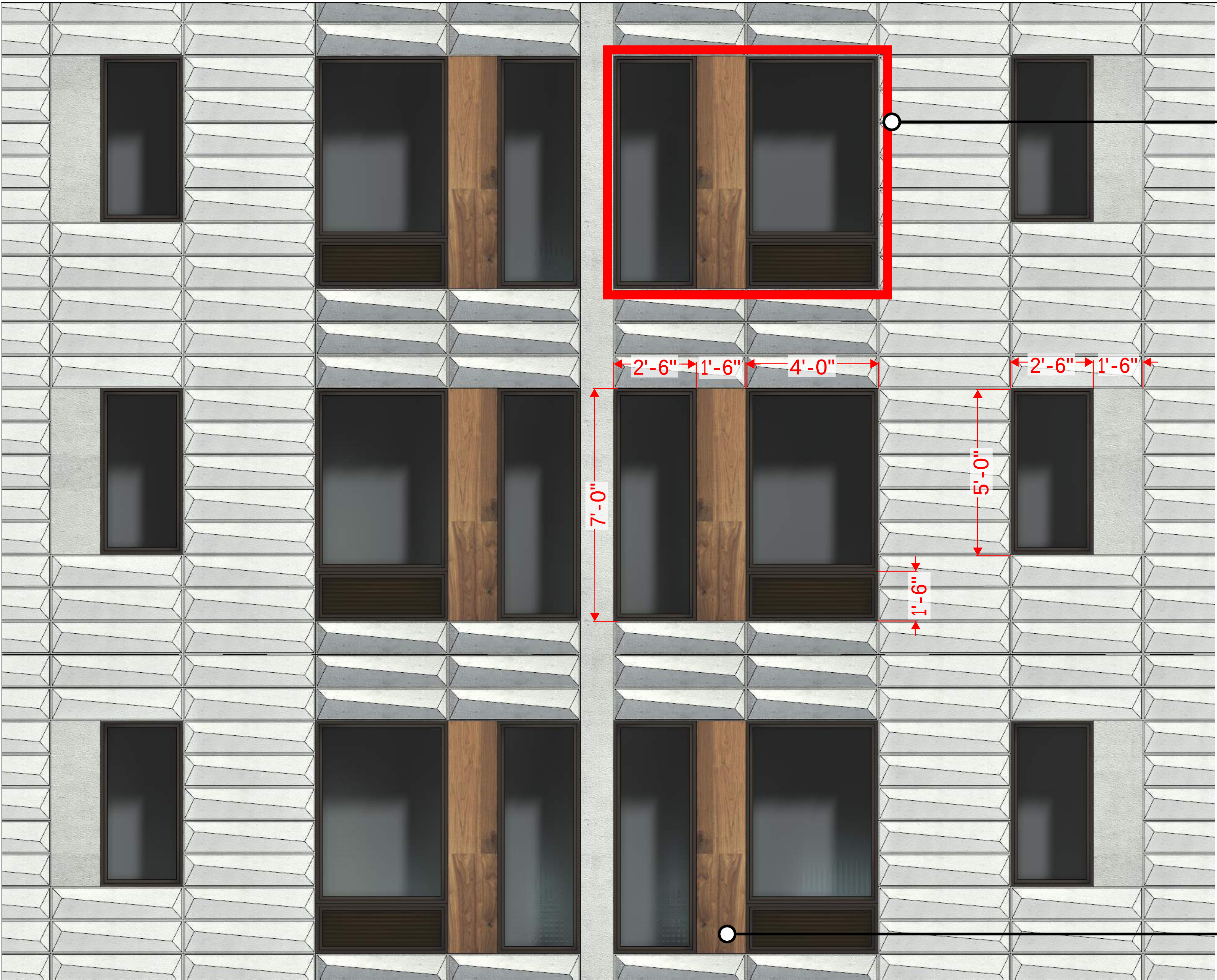
ENLARGED PARTIAL NORTH FACADE SHOWING TYPICAL WINDOW - LOUVER - LONGBOARD CONFIGURATION AND SIZES
