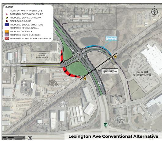
At-grade intersection, no new bridges required for this alternative. Railroad south of intersection if being investigated for potential high-speed rail.
