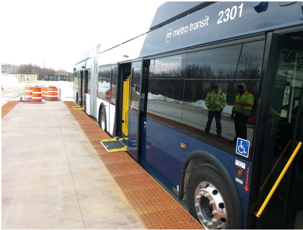
Figure 7-1: Transit Vehicle Using Bridge Plates on Vehicle Test Platform
