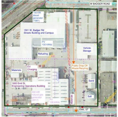
Figure 2 -- Satellite image of the site showing structures, functions, and existing solar PV arrays
