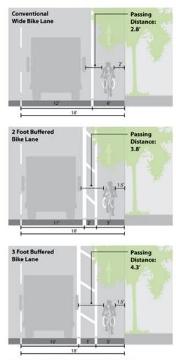
Measurements assume 10.5' vehicle width and 2' bicyclist width operating in the center of their lanes.
