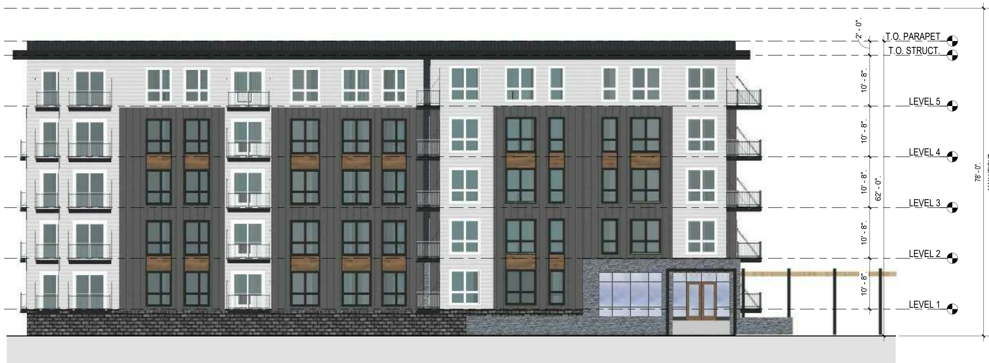
3 East Building - North Elevation A-8 1/16" = 1'-0"
