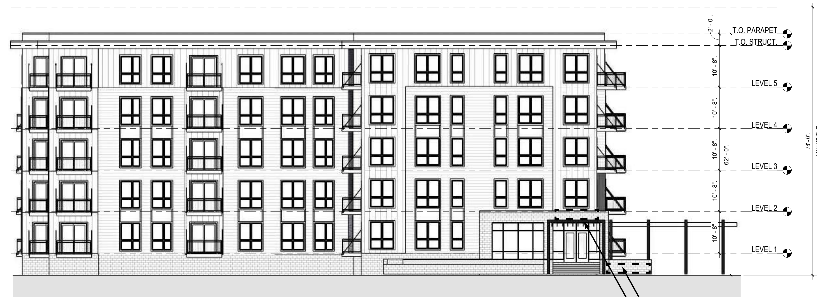
3 East Building - North Elevation A-8 1/16" = 1'-0"
