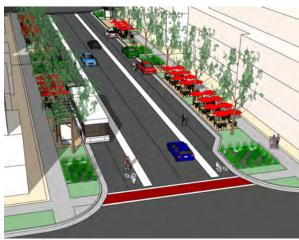
Odana Road, when extended, should feature buffered bike lanes, on-street terraces, 10 foot minimum terraces, and at least six foot sidewalks.
