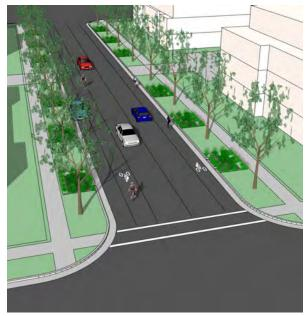
Charmany Drive should be extended west to connect with Normandy Drive. It should include on-street bike lanes. Westfield Road should be extended south from Mineral Point Road in a similar configuration as Charmany, but with parking on both sides of the street.
