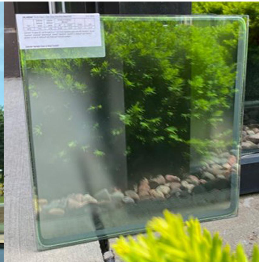
5 SOLARBAN 70 TRANSLUCENT GLASS SATINLITE 1 ON 3RD SURFACE (TO RECEIVE 2' X 4' BLACK BIRD GLAZING PATTERN)
