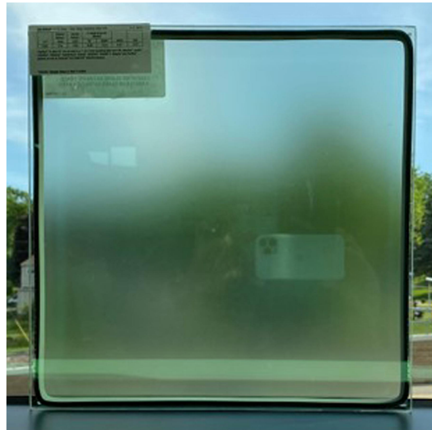
5 SOLARBAN 70 TRANSLUCENT GLASS SATINLITE 1 ON 3RD SURFACE (TO RECEIVE 2' X 4' BLACK BIRD GLAZING PATTERN)
