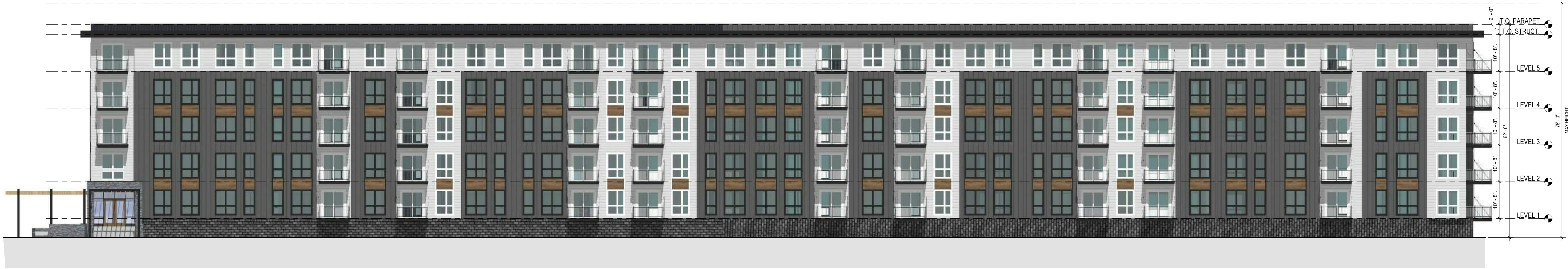
1 East Building - West Elevation A-8 1/16" = 1'-0"
