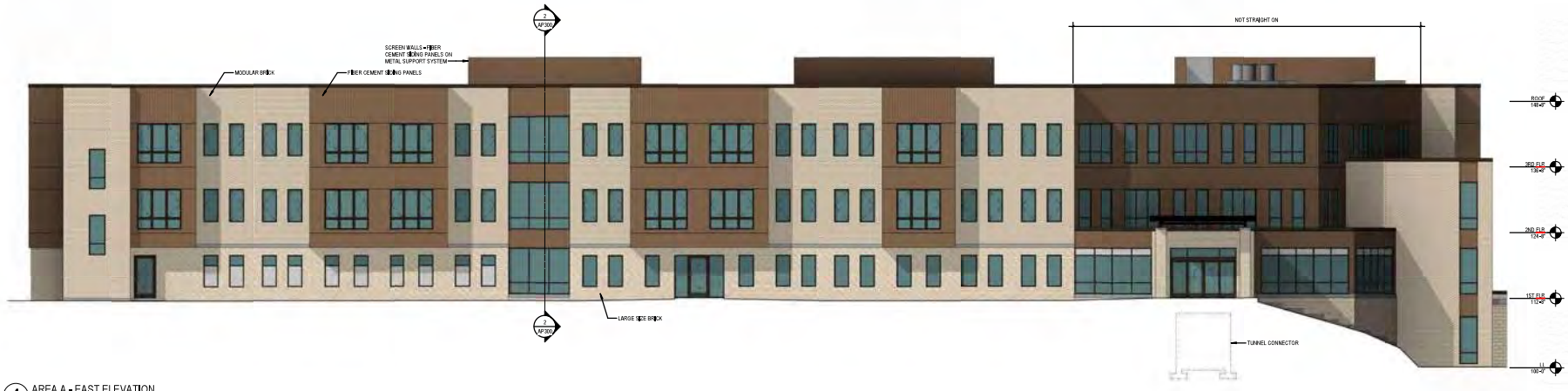
4 AREA A - EAST ELEVATION 1/8" = 1'-0"
