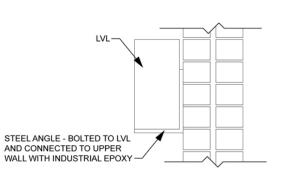
6 LVL WALL CONECTION EAST A300 Scale: 1/2" = 1'
