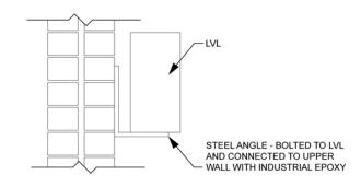
7 LVL WALL CONECTION WEST A300 Scale: 1/2" = 1'
