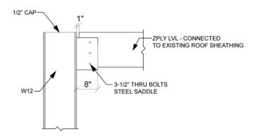
5 COLUMN LVL CONNECTION A300 Scale: 1/2" = 1'
