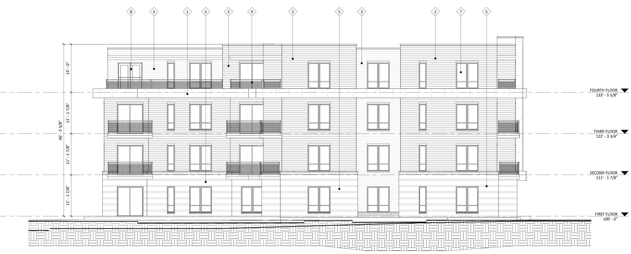
BUILDING ELEMENT (#1) - REVEAL COMPOSITE PANELS (#2) - 6" COMPOSITE LAP SIDING (#3) - 6" COMPOSITE LAP SIDING (#4) - REVEAL COMPOSITE PANELS COMPOSITE TRIM (#5) - STONE VENEER (#6) - CAST STONE BANDS & SILLS (#7) - COMPOSITE WINDOWS (#8) - ALUM. STOREFRONT CANOPY & BAY SOFFITS (#9) - RAILINGS & HANDRAILS
