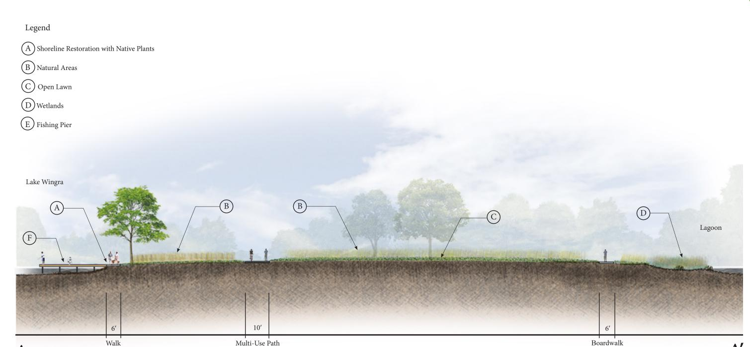
Figure 6.14. Vilas Park Drive and Peninsula Cross Section A-A' in Concept B
