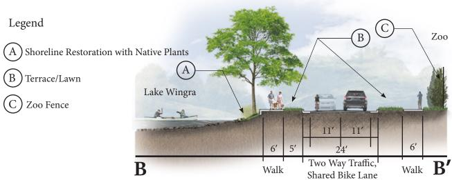
Figure 6.10. Vilas Park Drive Cross Section B-B' at the Zoo in Concept A
