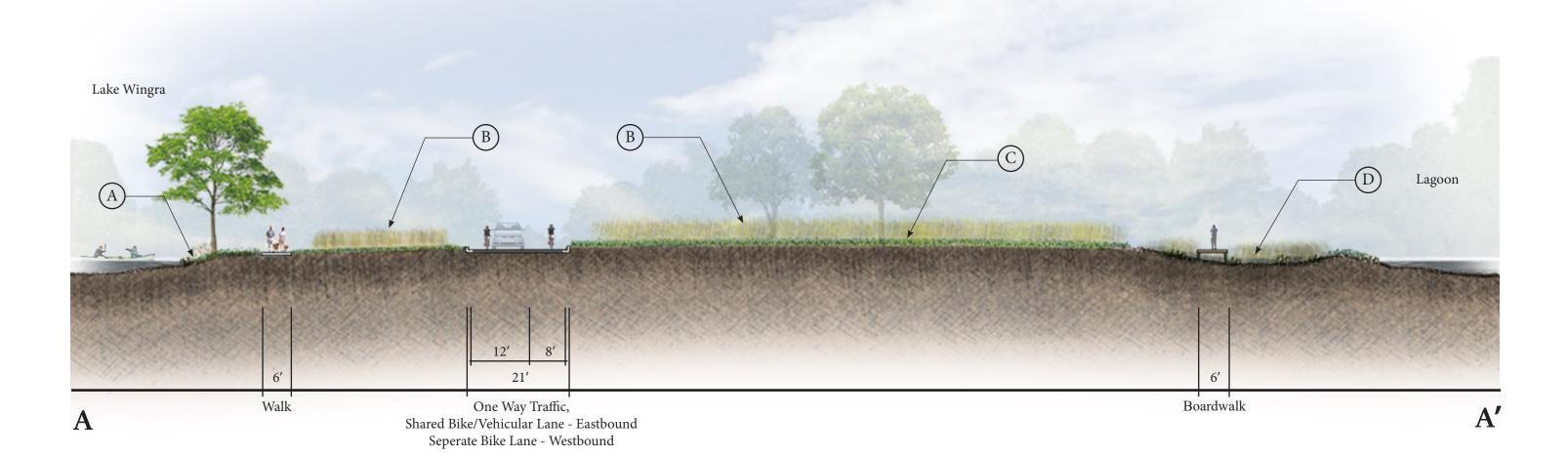
Figure 6.11. Vilas Park Drive and Peninsula Cross Section A-A' in Concept A
