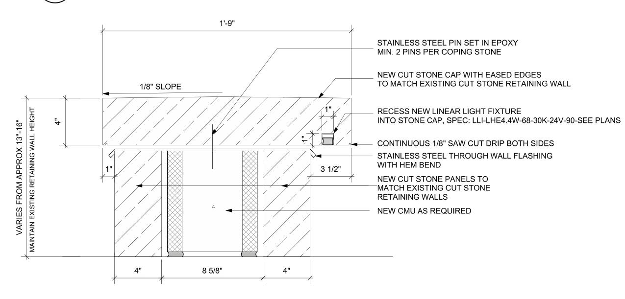
SECTION THRU NEW RETAINING WALL A1.1 | Scale: 3" = 1'-0"
