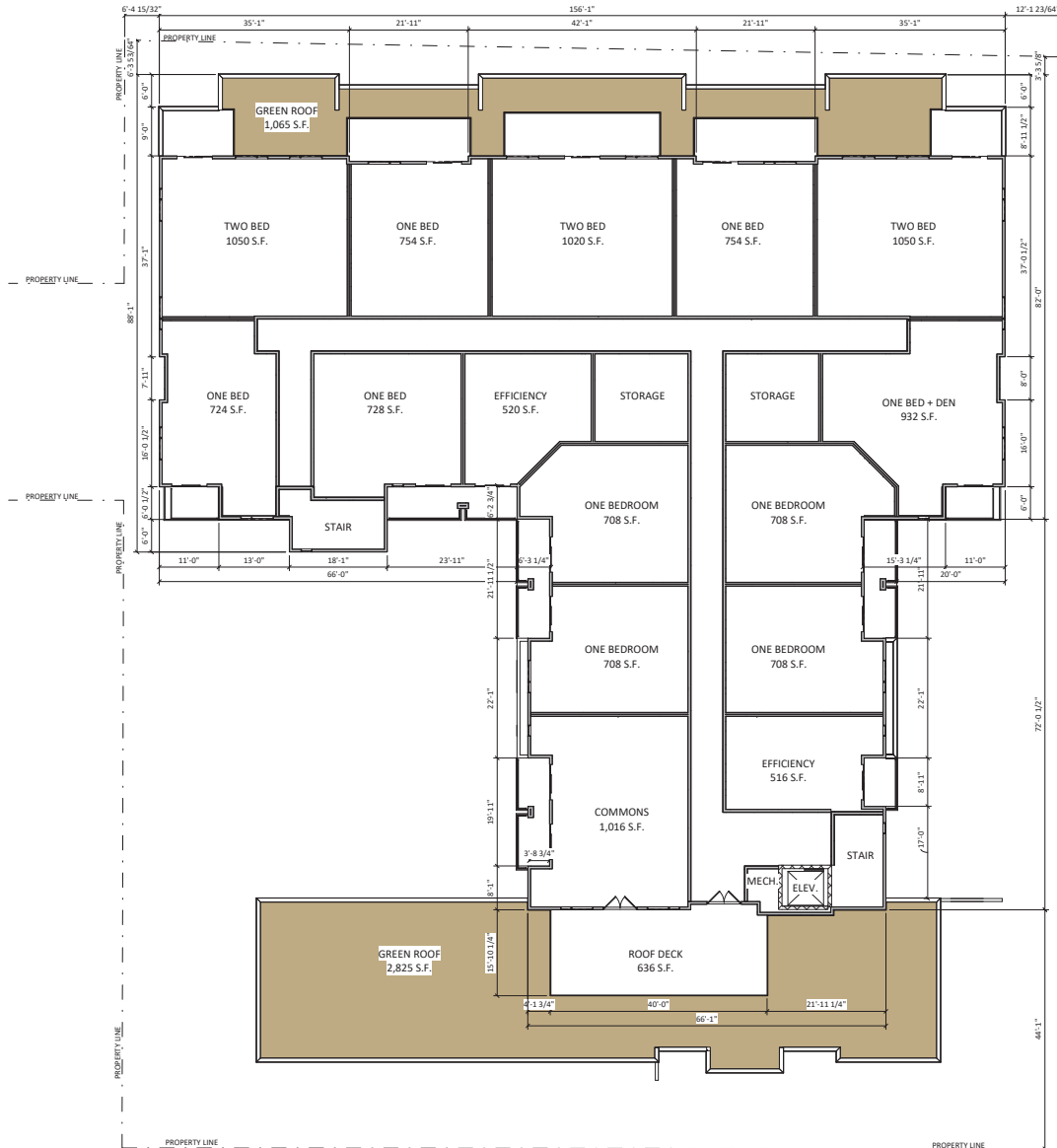
FOURTH FLOOR PLAN A-1.4 3/32" = 1'-0"
