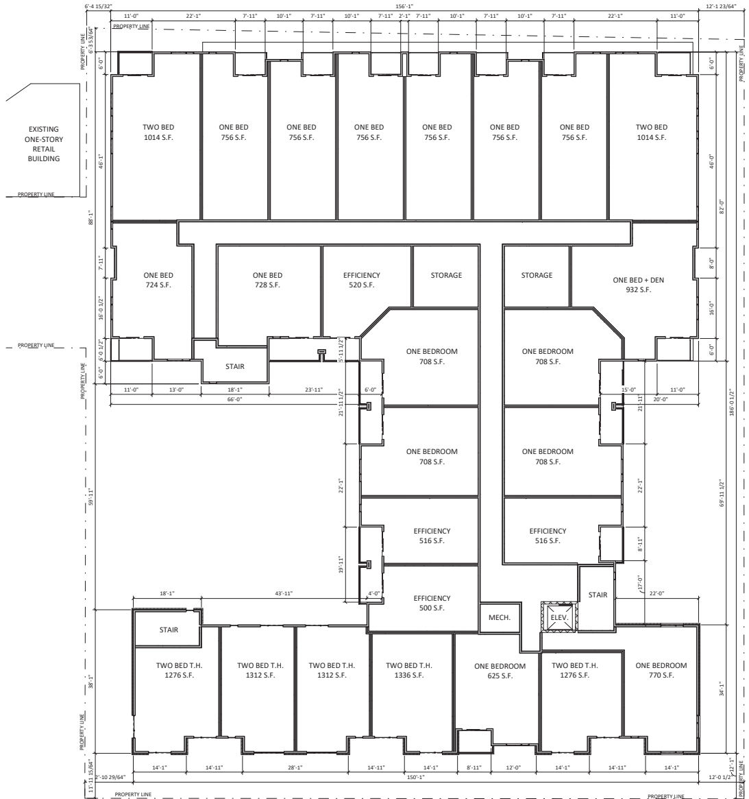
1 SECOND FLOOR PLAN 3/32" = 1'-0"
