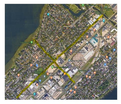
**Closure mechanism:** TBD by Transportation Engineering. We imagine that a single barricade located at each crossing intersection may be sufficient to prevent through traffic while maintaining vehicle access for emergency vehicles and residents of that blocks. Similar low-level signage and infrastructure has been successful for temporarily closing these streets during city race events, Breese Stevens events, and recent isthmus flooding emergencies.
