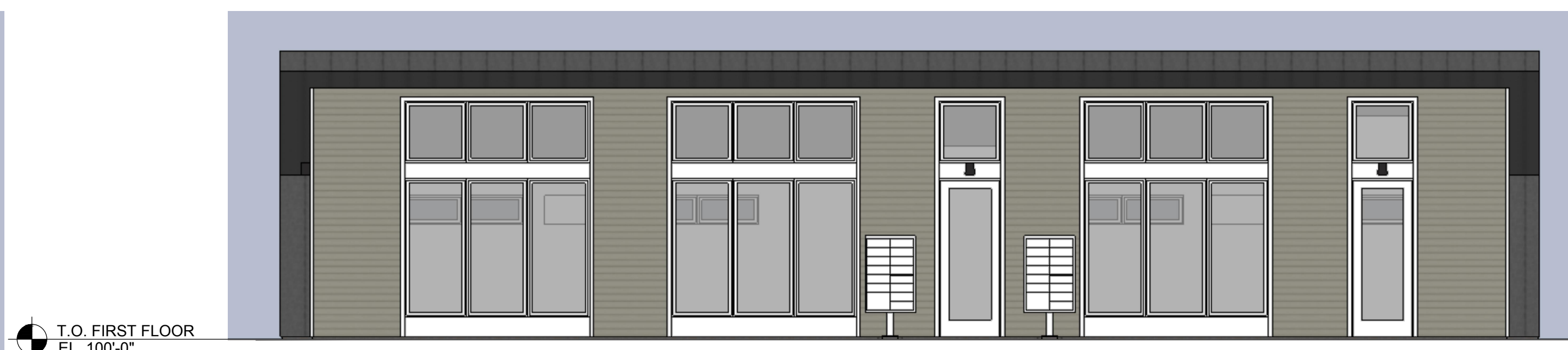
4 EAST ELEVATION - BIKE & FITNESS BLDG. A201a SCALE: 3/16"=1'-0"
