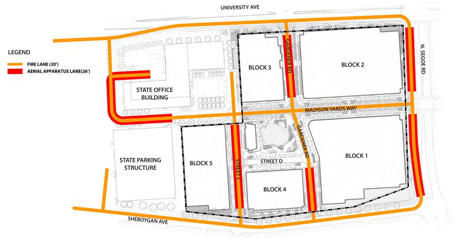
**FIGURE 12 - FIRE ACCESS DIAGRAM**
