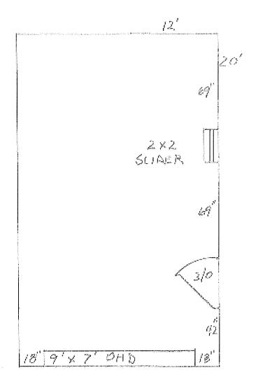
FLOOR PLAN 12' XZO ACCESSORY STRUCTURE 2106 F. MIFFLIN ST. BETH CANNESTRA 9.9.19 SCALE 1/4"=1'
