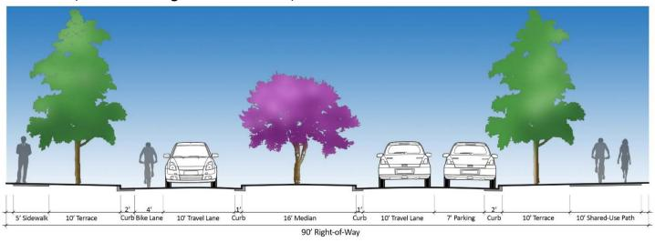
This alternate would replace the sidewalk and bike lane with a shared-use path on one side of the street. This would provide an off-street bike route alternative. Both sides of Burke are fronted with planned Housing Mix 1 development, which would likely mean an off-street path would have many single family home driveway crossings.
