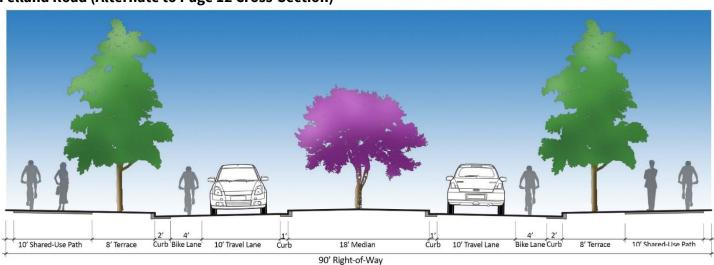
This alternate replaces the sidewalk along the right (east) side of the street with a shared-use path by expanding the right-of-way by five feet.
