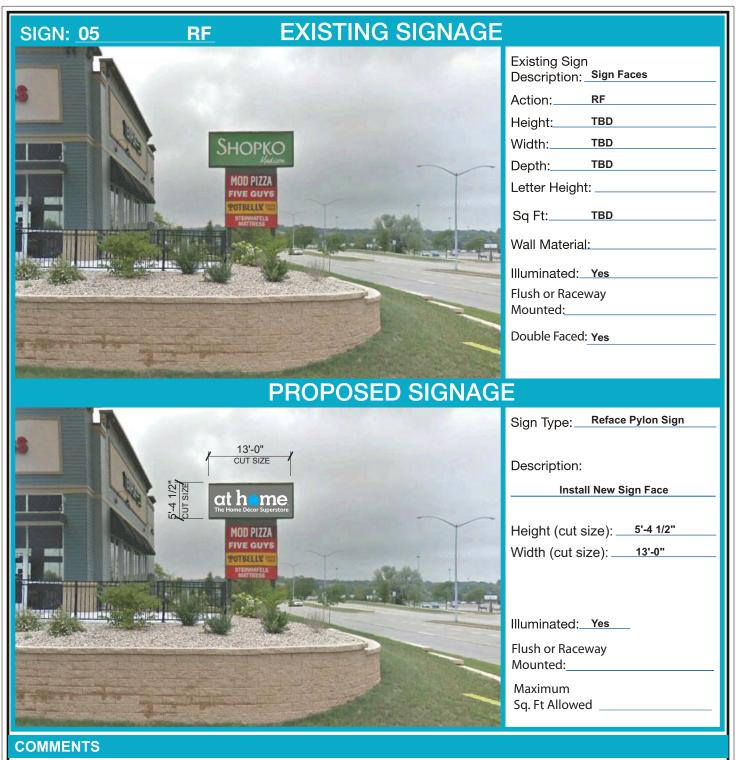
Copy change only to replace Shopko tenant panel with At Home tenant panel. Sign face of 3/16" flat polycarbonate with surface applied vinyl graphics. Sign is internally illuminated. Panel to be 5'-4 1/2" H x 13'-0" L.
