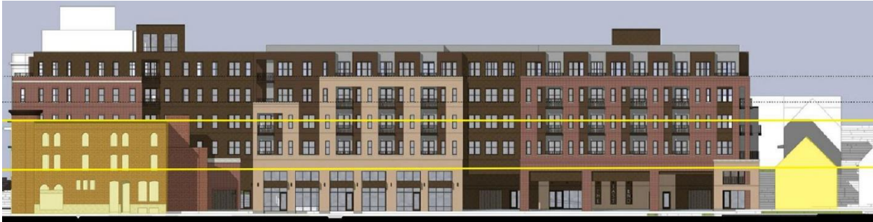
FIGURE 4. HEIGHT LINES OF ADJACENT STRUCTURES
