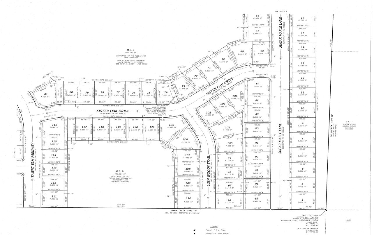
Placed 1-1/4" x 18" solid round iron rebar stake, weighing 4.30 lbs/ft. All other tot and outlot corners are marked with 3/4"x 18" solid round iron rebar stakes, weighing 1.50 lbs/ft.
