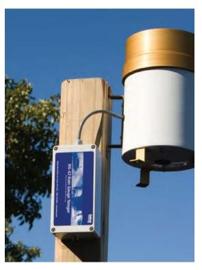
Tipping bucket rain gage with data logger Flush mount and pole mounted
