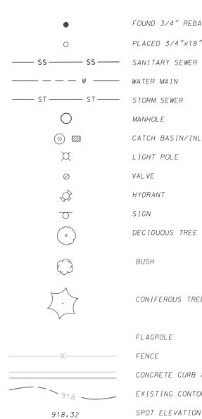
FOUND 3/4″ REBAR PLACED 3/4″×18″ REBAR (WT=1.5 LBS/FT) MANHOLE CATCH BASIN∕INLET LIGHT POLE VAL VE HYDRANT SIGN DECIDUOUS TREE
