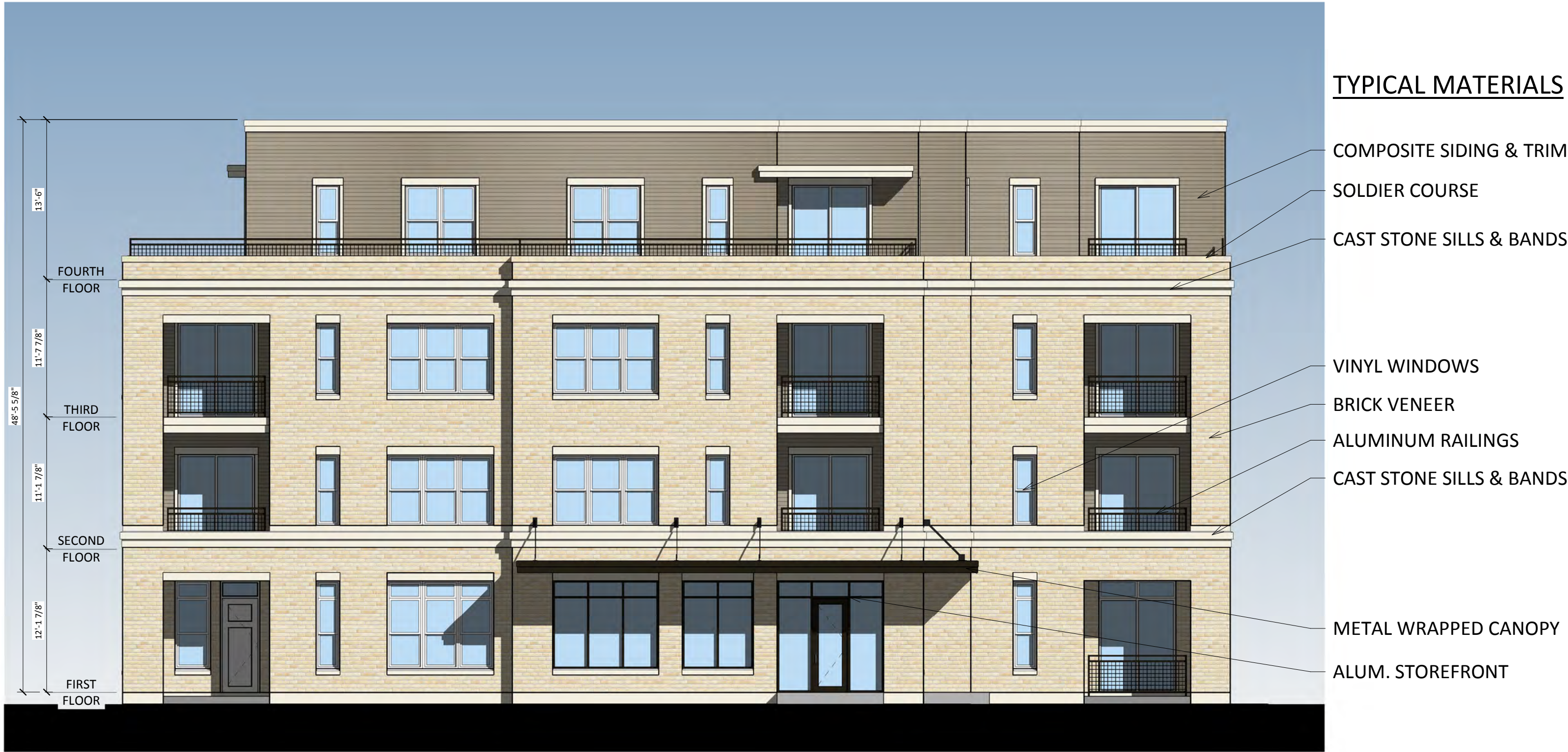
1 A-2.3 SOUTHEAST ELEVATION - ALONG E. WASH - RENDERED 1/8" = 1'-0"
