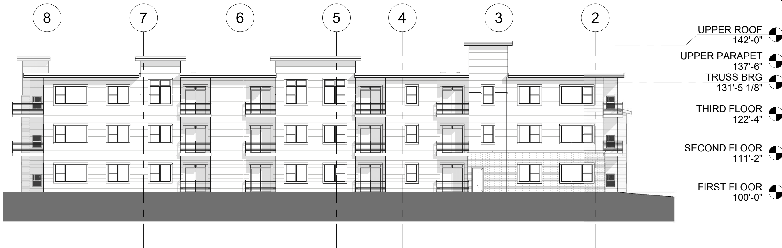
① NORTH BUILDING ELEVATION-UDC 1/16" = 1'-0"
