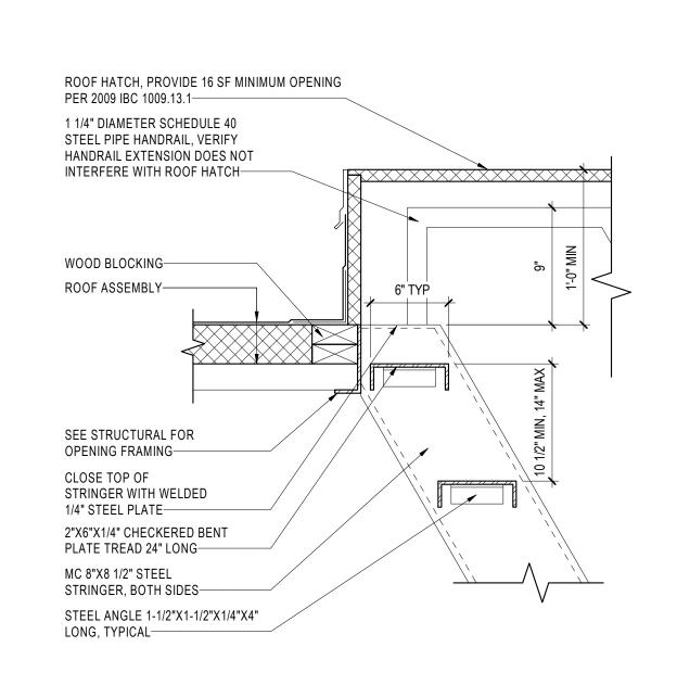
1C SECTION DETAIL - SHIP'S LADDER AT ROOF HATCH
