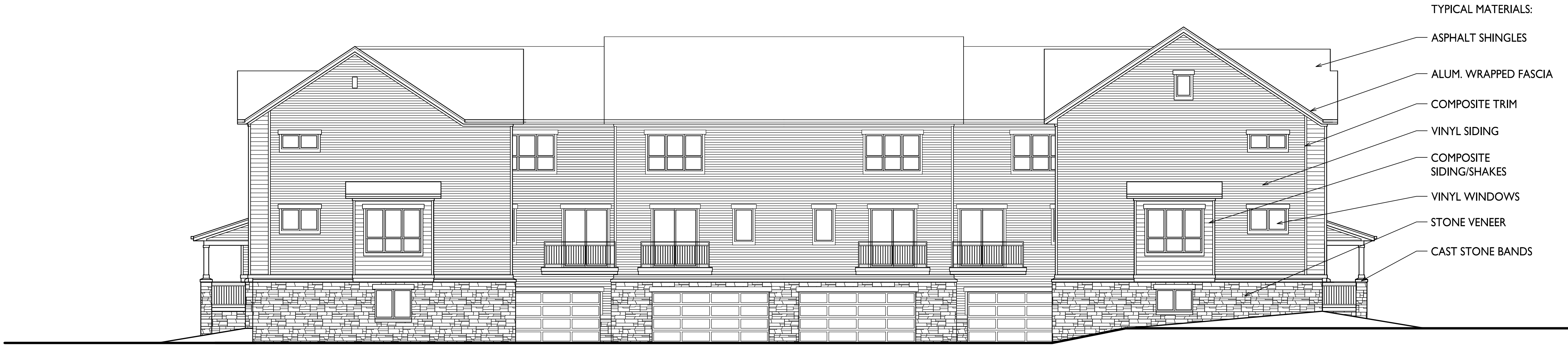
1 EAST ELEVATION A-2.2 1/8"=1'-0"
