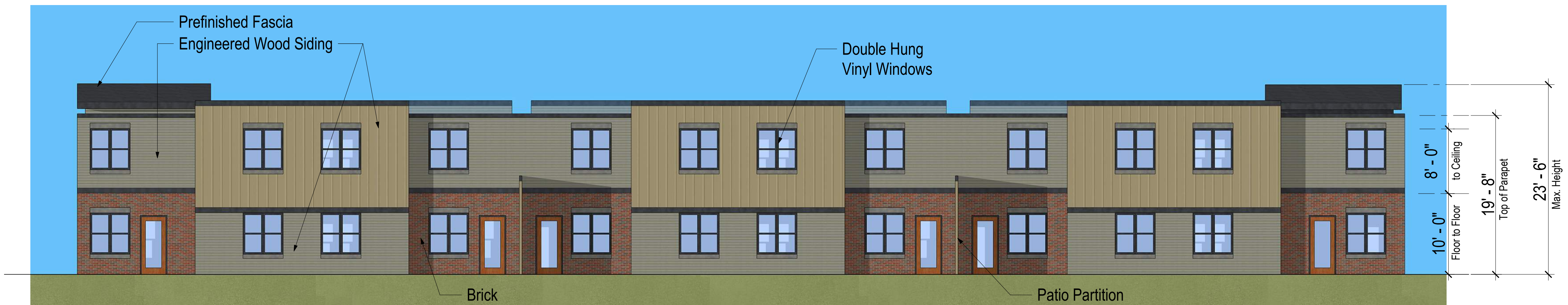
1 North Elevation - Townhouses w Garages 1/8" = 1'-0"
