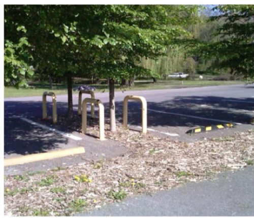
Parking lot near flood control channel. No catch basins, pipes, or outfalls are required. No negative impact on surface water quality due to parking lot. Trees can thrive while more space is devoted to parking spots, resulting in a smaller overall footprint for the parking lot.
