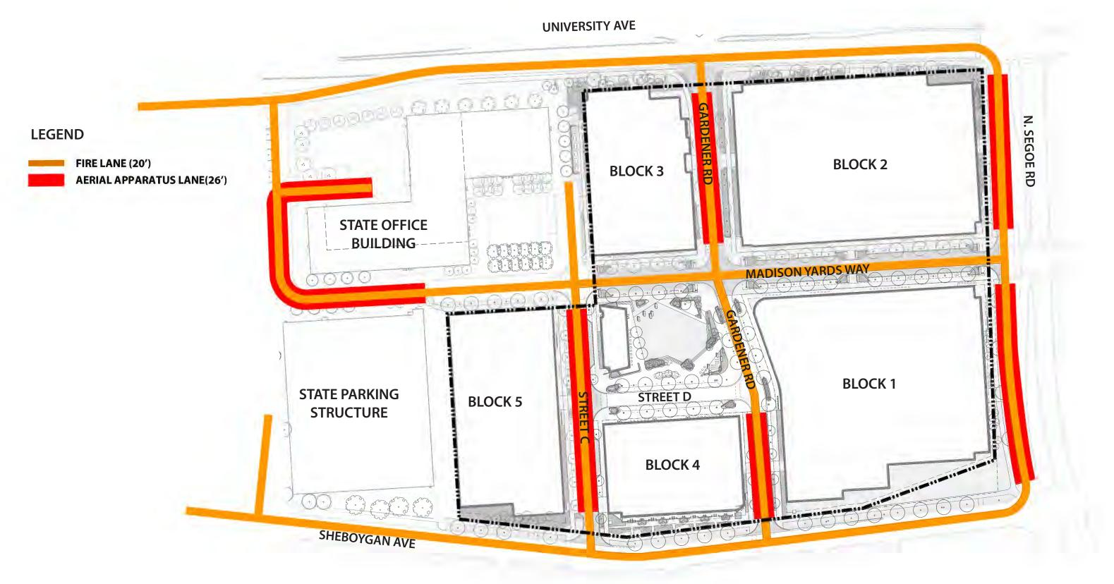
**FIGURE 12 - FIRE ACCESS DIAGRAM**
