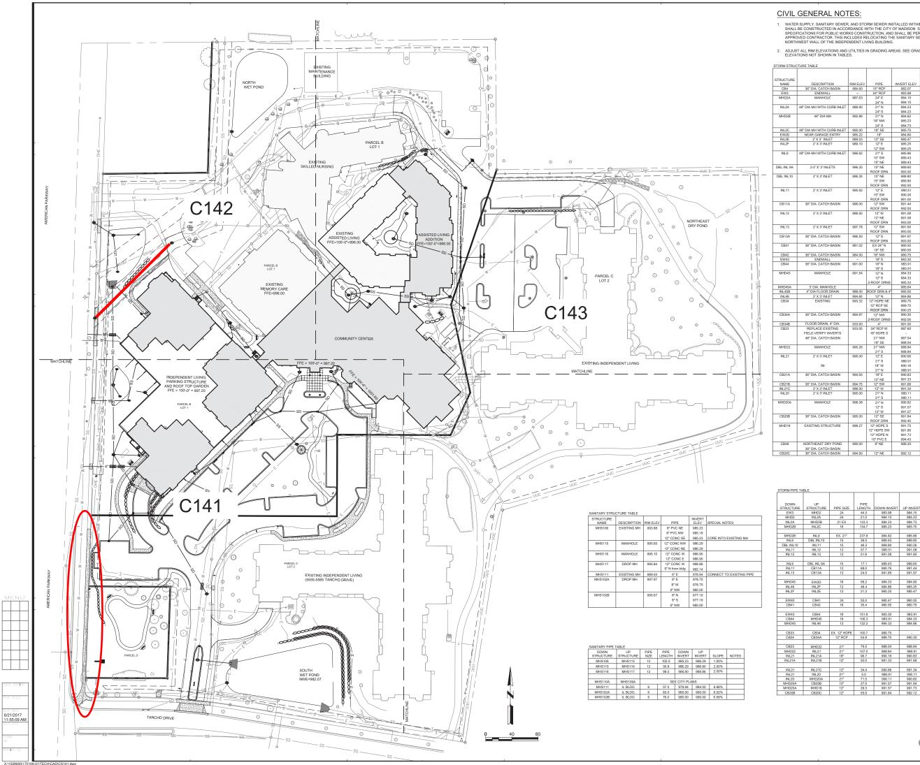
WATER SUPPLY, SANITARY SEWER, AND STORM SEWER INSTALLED WITHIN THE RIGHT-OF-WAY SHALL BE CONSTRUCTED IN ACCORDANCE WITH THE CITY OF MADISON STANDARD SPECIFICATIONS FOR PUBLIC WORKS CONSTRUCTION, AND SHALL BE PERFORMED BY A CITY APPROVED CONTRACTOR. THIS INCLUDES RELOCATING THE SANITARY SEWER ALONG THE NORTHWEST WALL OF THE INDEPENDENT LIVING BUILDING.
