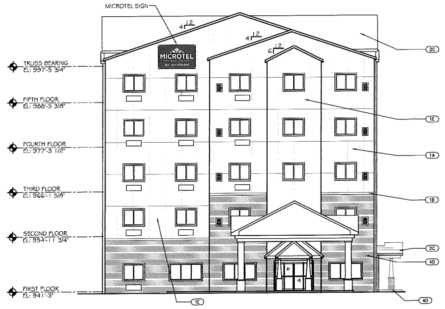
3 EAST ELEVATION w/ PORTE COCHERE SCALE: 3/32"=1'-0"
