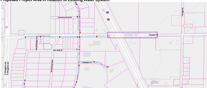
**Project Scope:** Extend new transmission line water mains along Hoepker Rd. from the existing water main west of the Interstate 39/90/94 bridge, to approximately 1,500-FT east in order to provide service to development within the Pumpkin Hollow Neighborhood area.
