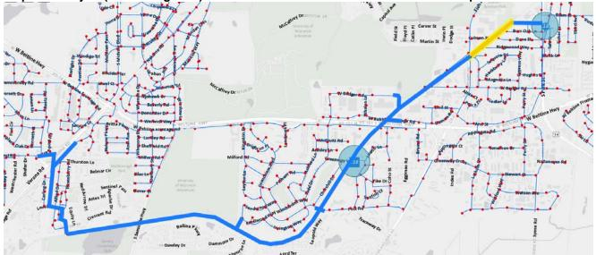
**Project Scope:** Proposed installation of approximately 2,400-FT of new 12-IN water main along the WisDOT railroad corridor located between Fish Hatchery Rd and North Ave in the City of Madison and Town of Madison. This is the final phase of a 5-mile transmission line and pump station project which connects Unit Well 18 to Pressure Zone 7 in order to improve system hydraulics, redundancy and fire flow capacity along this transmission corridor.
