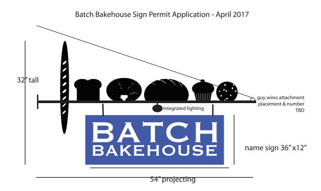
2x2 inch tubular steel welded to a heavy duty mounting plate ustom universal straight arm bracket with 6 steel waterjet cut 1/4" thick bread shapes welded to top of main arm (french bread to be welded to top & bottom). Mounting bracket 6x6" with 4 - 3/8" thru holes for mounting. Color/Finish: textured black powder coat. Two 1.5" OD steel bracket rings mounted to bottom of arm for hanging name sign. 2 Guy wire rings for added support.
