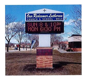
The **existing** freestanding sign is  $5'-0" \times 8'-0" - 40/80$  sf2 including the "peak". The overall height of the sign is 12'-0".
