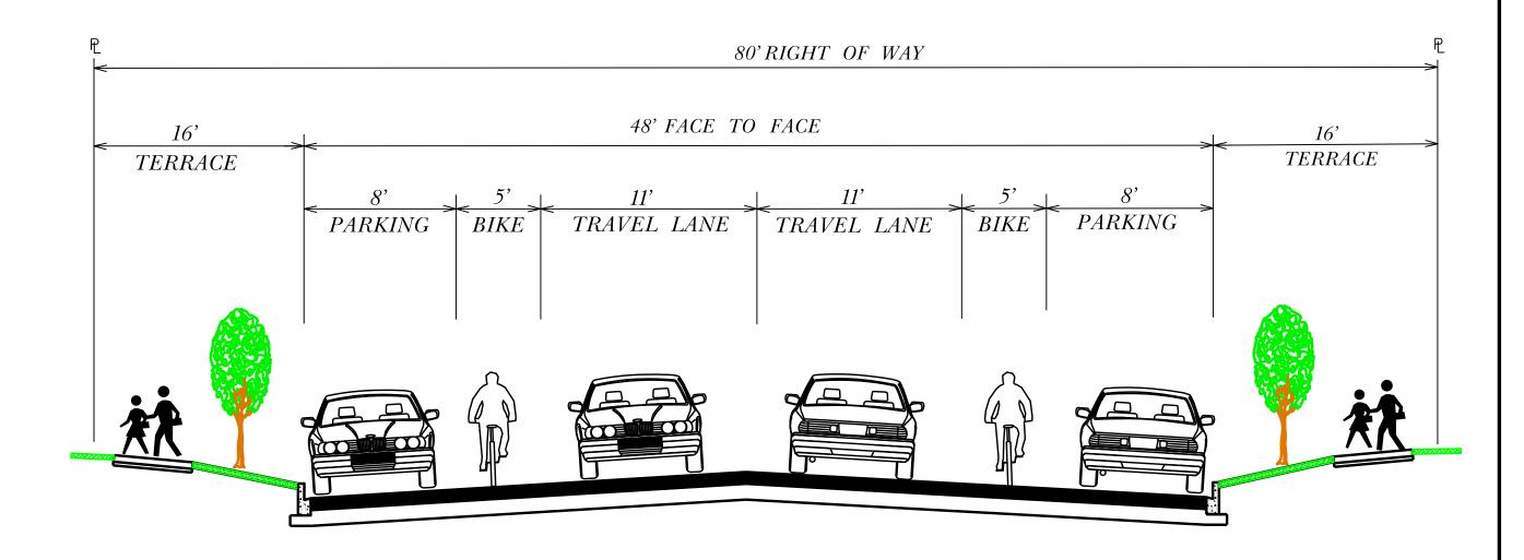
TYPICAL FINISHED SECTION WATTS ROAD
