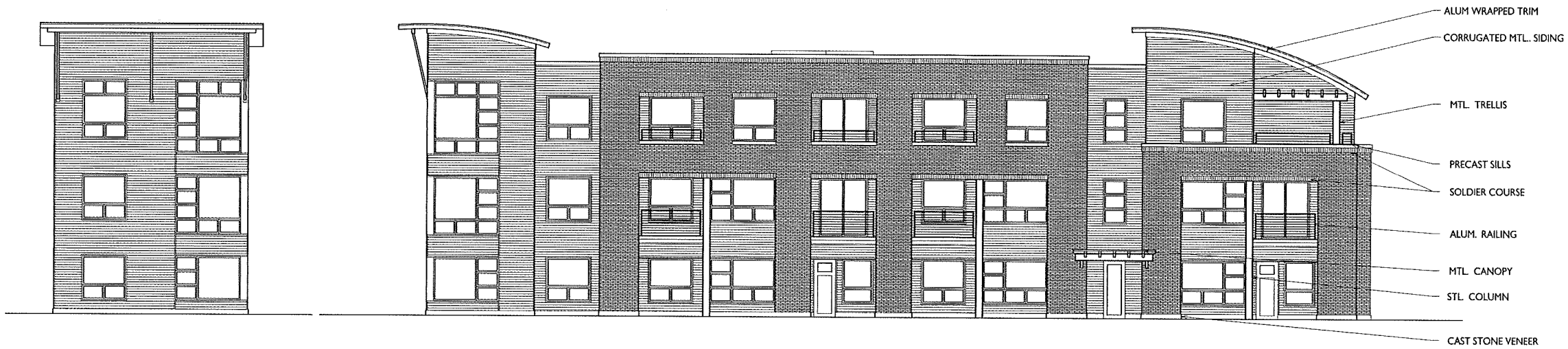
1 Elevation along Eastwood Drive A-2.1 1/4"=1'-0"
