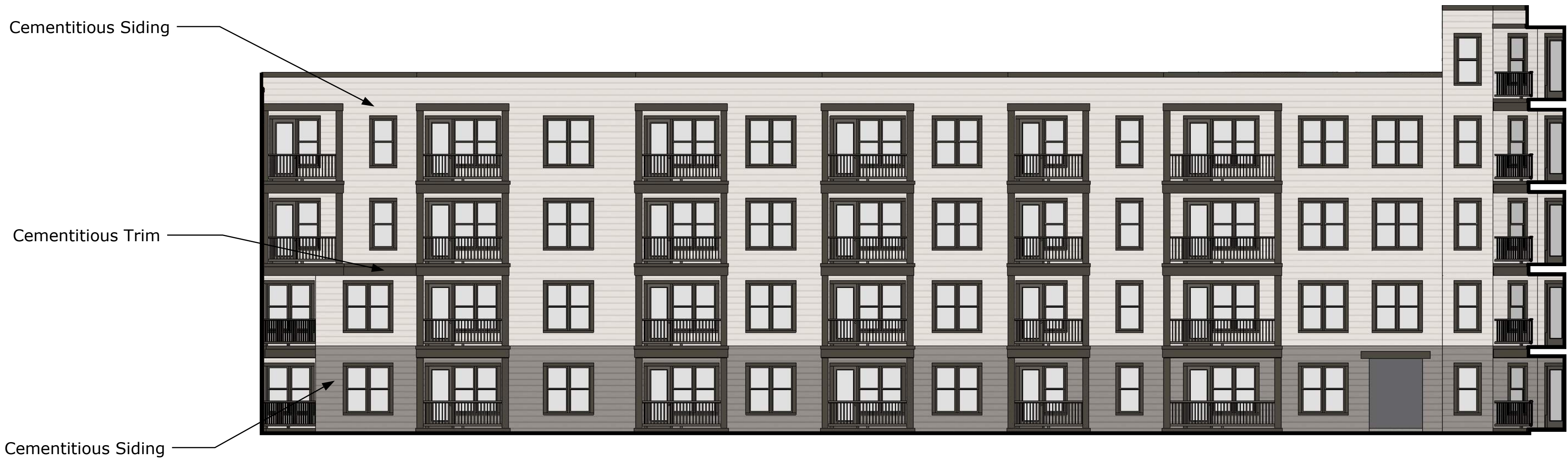
1 Interior Courtyard - North Elevation Scale: 3/32" = 1'-0" Elevation
