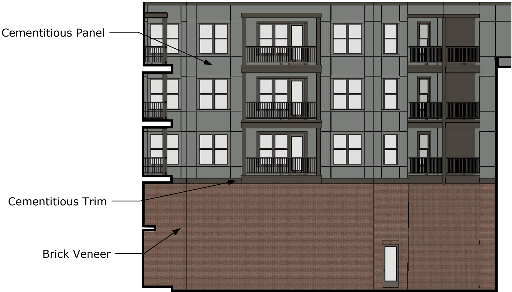
3 River Courtyard - East Elevation Scale: 3/32" = 1'-0" Elevation
