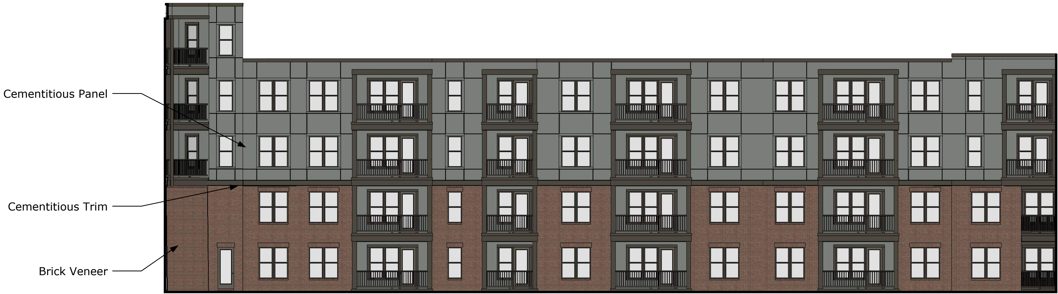
2 River Courtyard - South Elevation Scale: 3/32" = 1'-0" Elevation
