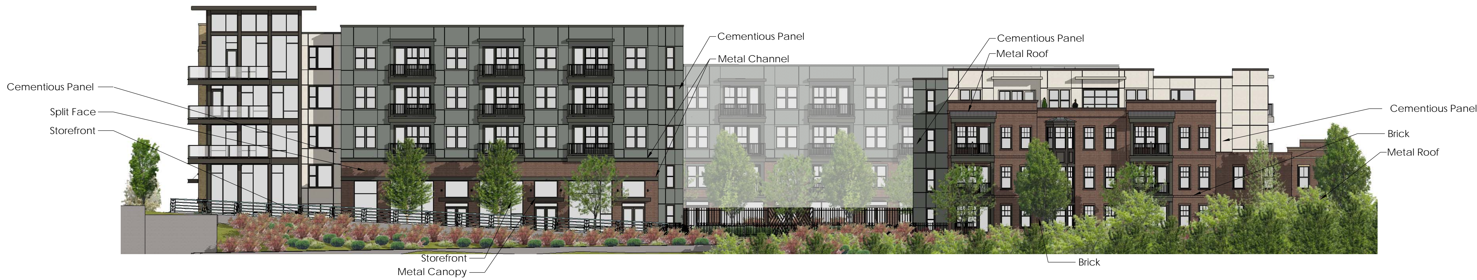
2 River Elevation - Option 2 Scale: 1/16" = 1'-0"
