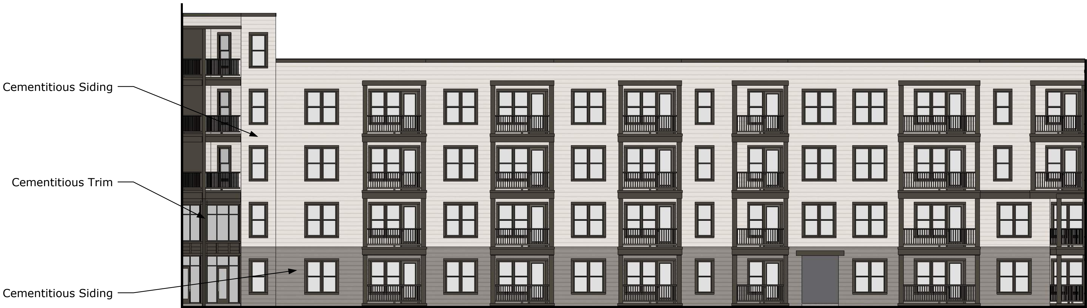
2 Interior Courtyard - South Elevation Scale: 3/32" = 1'-0" Elevation
