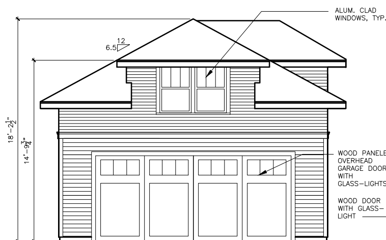
GARAGE FRONT ELEVATION (EAST)
