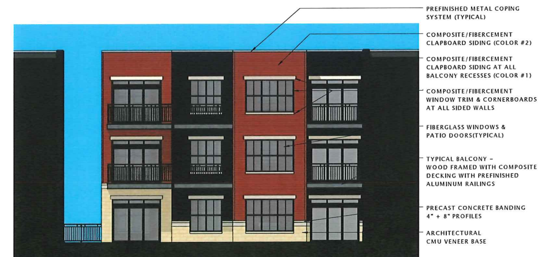
⑩ COURTYARD ELEVATION (NORTH) 1/8" = 1'-0"
