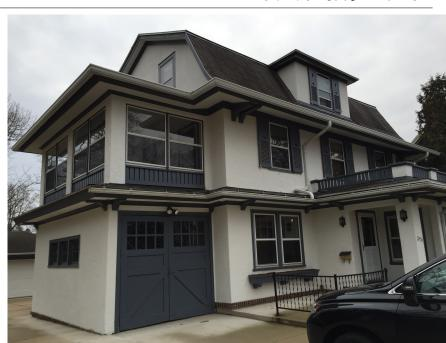
FRONT PORCH: REMOVE WINDOWS. MODIFY COLUMNS AND RAIL -PAINTED CEDAR COLUMNS. CEDAR RAIL TO MATCH ORIGINAL PARAPET DESIGN. REMOVE PARAPET RAIL AND **RESTORE ROOF TO ORIGINAL** CONDITION (CURRENTLY HAS A LOW PITCH BUT THERE IS SOME STRUCTURAL EVIDENCE THAT IT WAS PARTIALLY FRAMED OVER A FLAT ROOF, - VERIFY AT DEMO). MAINTAIN CORBELS AND CROWN.
