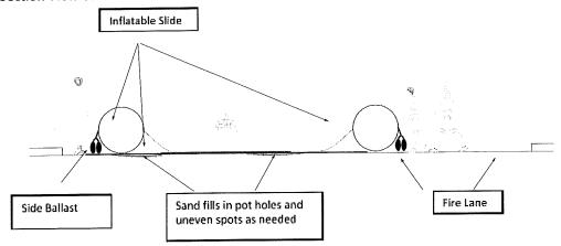
i) Ballast will be per engineering specifications; typically sand bags are sufficient, especially given the weight of the water in the system. If greater ballast is specified, we will use precast concrete block or water-filled barriers.
