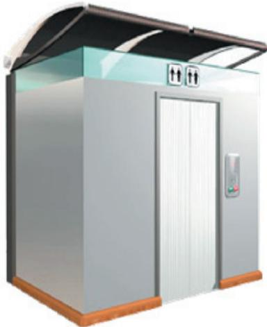
APTs vary in design based on manufacturer and city, but are generally made of regular and enamel-coated steel, porcelain, and aluminum. Push-button doors open automatically after a set time period, usually 10-15 minutes. After each use, the unit is sprayed with disinfectant, rinsed with high power jets, and dried. The cleaning cycle usually lasts about five minutes.
