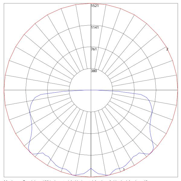
Maximum Candela = 1521 Located At Horizontal Angle = 0, Vertical Angle = 45 # 1 - Vertical Plane Through Horizontal Angles (0 - 180) (Through Max. Cd.) # 2 - Horizontal Cone Through Vertical Angle (45) (Through Max. Cd.)
