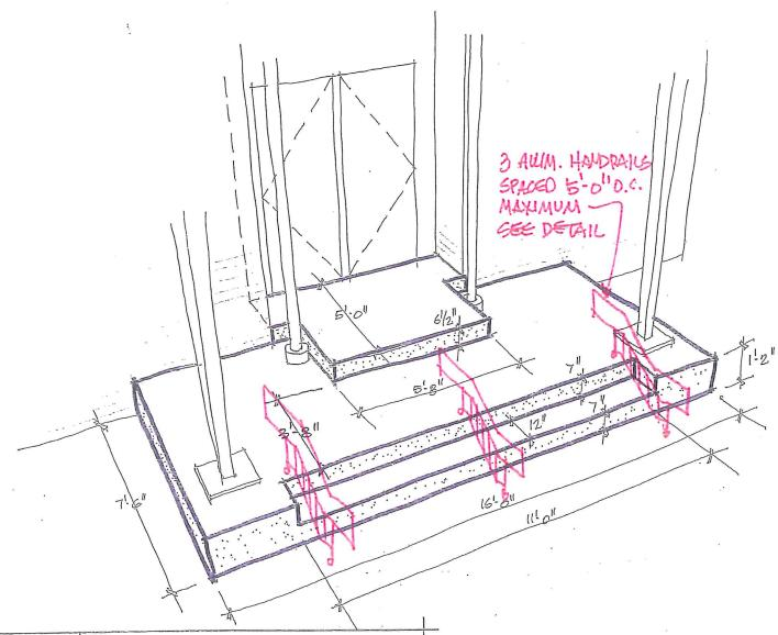
REMOVE & REPLACE EXISTING CONCRETE ENTRY STOOP - EXTEND TOP STEP AT DOOR SILL AG SHOWN, REMOVE & REPLACE EXISTING CANOPY SUPPORTS & LIGHT POLES
